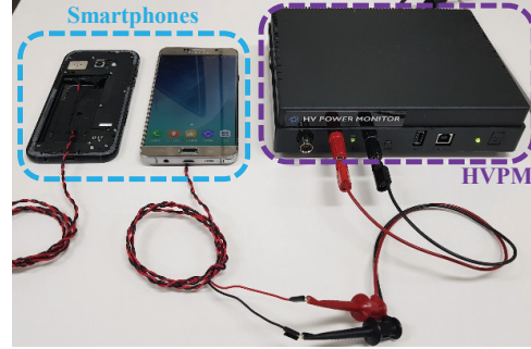
Figure 15. Our experimental setup to measure the energy consumption of mobile SoCs
